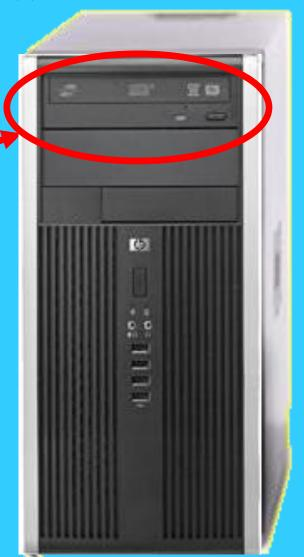
The **Power Switch** turns just the computer on and off, NOT the monitor.
