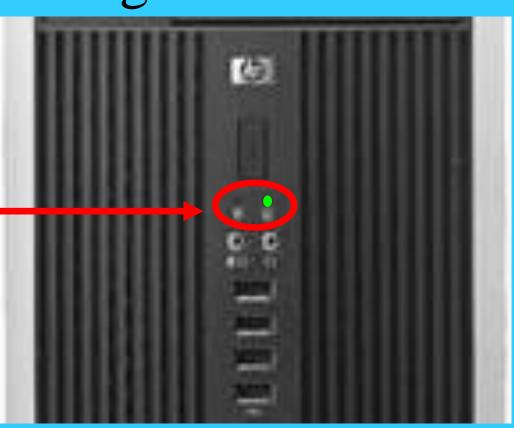
This is the hard drive light. When on, this light just tells us that the computer is doing some action that you told it to do, such as opening a program or saving a file.
